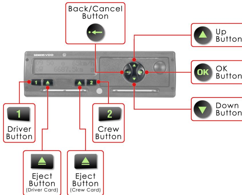
Below the main display are the Driver button ('1') and the Crew button ('2'), which are used to select the appropriate activity mode for the driver or crew member. Adjacent to each of these is an 'Eject' button for the relevant slot. If a Driver Card is inserted in either the driver or crew slot, the associated button is only active when the ignition is switched on and the vehicle is stationary.
