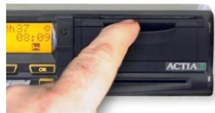
The cover will drop down on a hinge and a red piece of plastic will then be visible. Pull the red plastic out to the front of the cassette drawer and place a new print roll onto it. Push the front of the plastic back into the cassette drawer with the print roll on top of it, then lift up and close the cassette front. Ensure that the loose end of the print roll is drawn out over the top of the cassette drawer front when it has been latched back into place. The VU printer is now ready for use.
