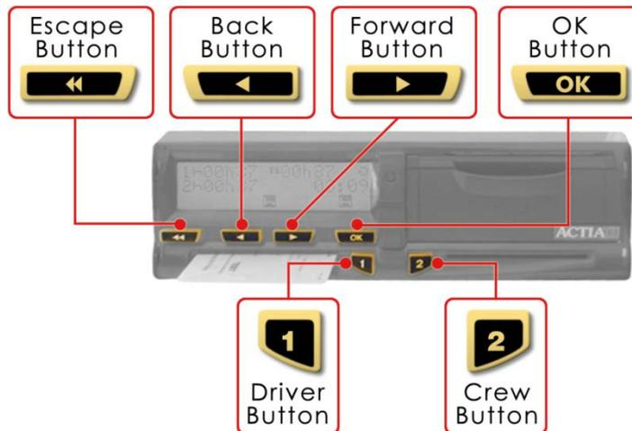
To the right of 'slot 1' is the Driver button ('1') which must be pressed and held to enable the insertion and withdrawal of the driver's card. Similarly, there is a single Crew button ('2') to the left of 'slot 2' which allows a crew member to insert or withdraw their card.
